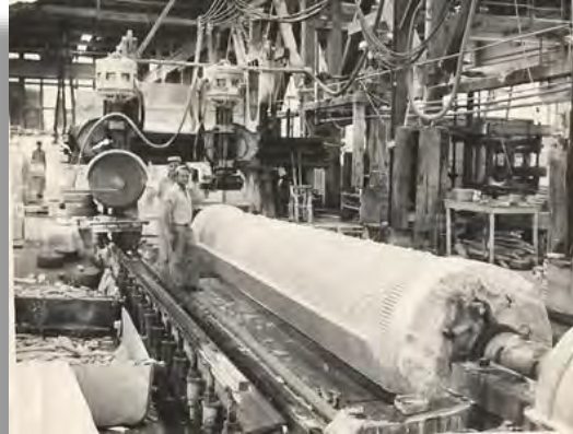
Figure 26: Marble Lathe inside Blue Ridge Marble Co.
